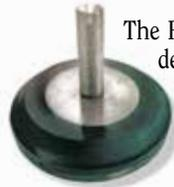
The RoughDeck was engineered to use a steel and neoprene sandwich design called SUREFOOT. A steel cup sits on the floor and is bonded by a pliable neoprene cushion to a steel top plate with attached threaded stem. This pliable sandwich allows the stem and top plate some plasticity to move laterally and tilt independently of the bottom steel cup. This allows the foot to accommodate small deflections and uneven floors.
