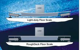
The exaggerated figure illustrates the problems of deck and load cell deflection. The RoughDeck design minimizes deflection of the deck and feet.
