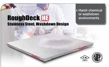
The RoughDeck HE is a hostile environment, stainless steel floor scale designed specifically for corrosion resistance and long life in demanding washdown applications. Design features include a 6", 304 stainless steel channel frame and smooth top plate. The RoughDeck HE comes standard with four stainless steel, IP67 welded seal, shear beam load cells, four stainless steel surefeet, a stainless steel NEMA4X
