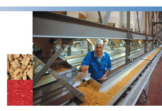
Precise feeding of process materials is often critical to maintaining product quality. A feeder that weighs accurately and reliably can reduce material waste, help maintain blend consistency and increase profits.
